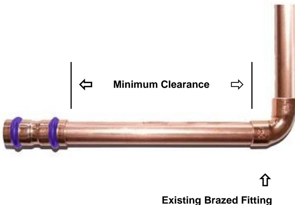
**Brazing close to EZIPRESS™ fitting joints** should be avoided as the heat generated by the process can damage the seals of the fitting. To ensure that damage is not caused, the minimum clearances in the following table should be observed. It's also recommended that additional heat suppression methods are employed to prevent damage to the joint.
