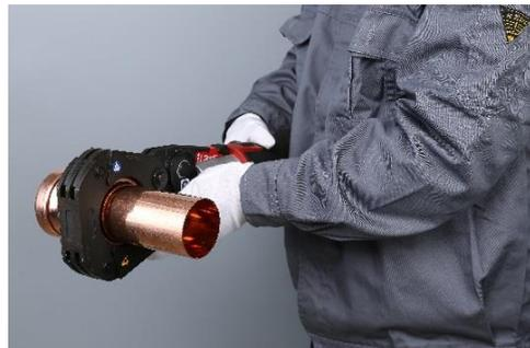
Depress tool trigger until pressing operation is completed fully. Also, refer to manufacturer’s instructions for specific details on the operation of their tool.
